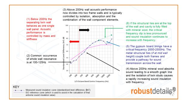
Typical airborne sound insulation graph features are shown in this slide.
