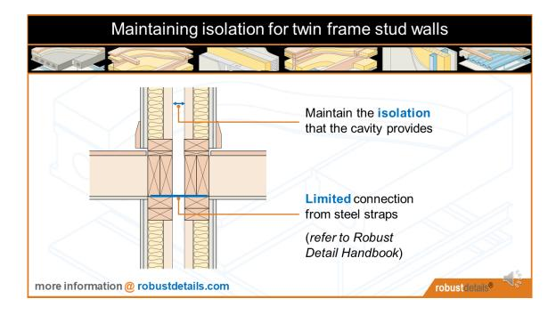
The cavity of these separating walls provides the isolation, or separation between the dwellings on either side – so it's important for the isolation to be maintained.
