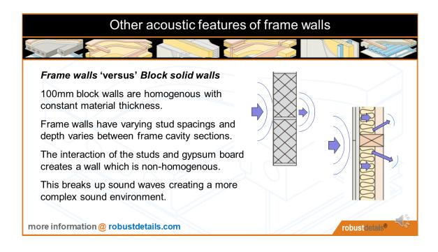
Unlike standard 100mm block walls which are quite uniform, fairly homogenous and of constant material thickness, frame walls have studs at various spacings, and the wall depth varies between the frame and cavity bay sections.
