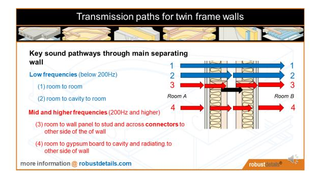
Sound transmission through timber or metal twin frame separating walls behaves differently at low, mid and high frequencies.
