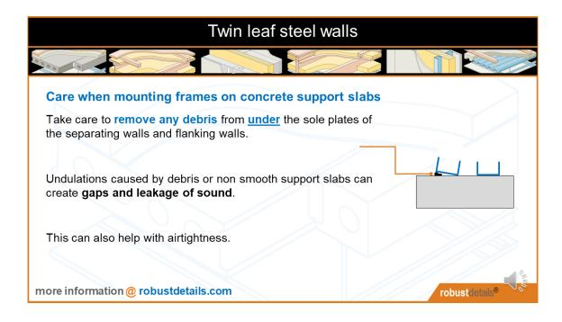
Care should be taken when mounting frames on concrete support slabs
