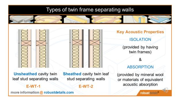
There are 2 primary types of twin timber stud separating walls, these are Unsheathed and Sheathed.
