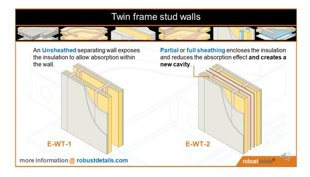
Using an **Unsheathed** separating wall exposes the insulation to allow for absorption in the main wall cavity.
