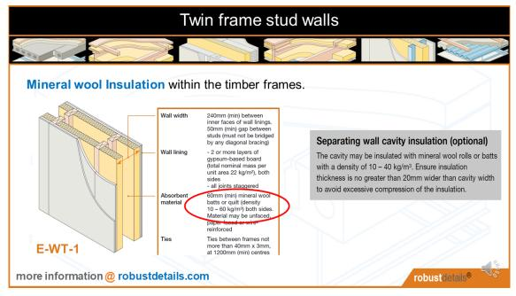
Mineral wool insulation can absorb sound that gets into the frame and eliminates reverberation.
