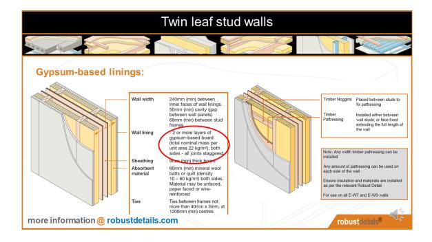
For all light frame separating wall Robust Details specify a minimum of 2 layers to give a minimum mass per unit area of 22kg/m<sup>2</sup> on both sides. And it's critical this is followed.
