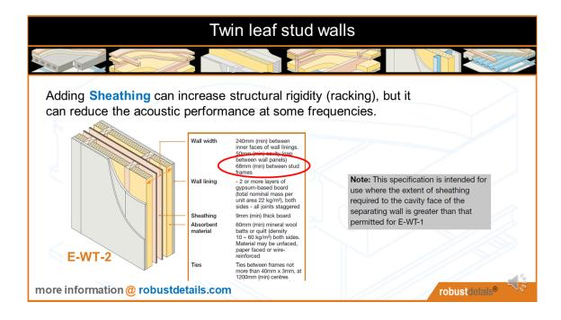
If more sheathing is required, including the panels being fully sheathed, then E-WT-2 needs to be used.
