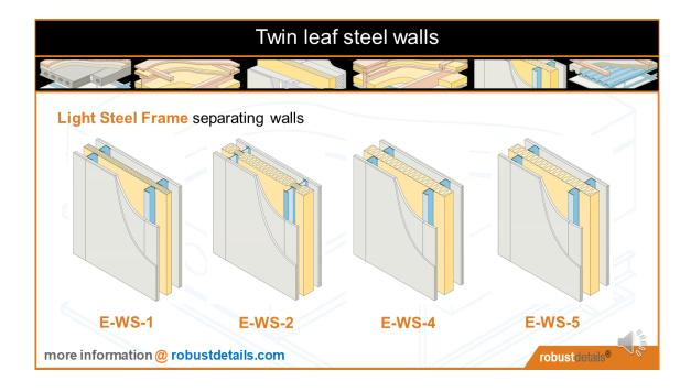
As can be seen, the steel walls are all very similar in design, albeit the specifications of the insulation and gypsum board does vary from one Detail to the next.
