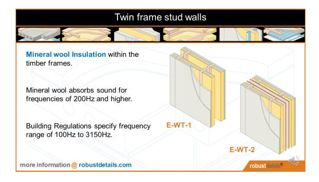
The absorption materials such as mineral wool play an important acoustic feature as the material is able to absorb sound from 200Hz onwards.
