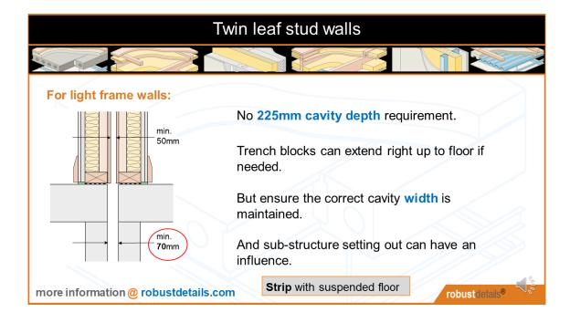
So even though there's no depth requirement, we still need the right width. It is possible to use the substructure as a setting out guide for the timber frames. EWT1 requires 50mm between frames, so substructure is drawn up with a corresponding 50mm.
