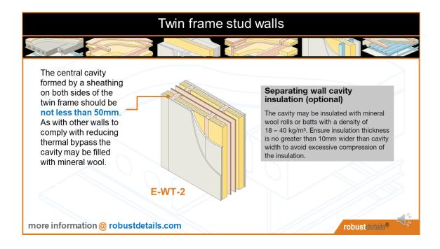
The central cavity formed by a sheathing on both sides of the twin frame should be not less than 50mm.
