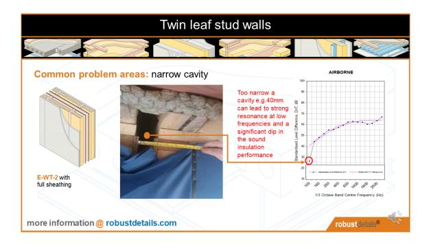
If the cavity is too small – this example shown measures 40mm, there will invariably be a dip at 125hz, as panel resonance starts up – and this could lead to test failure.
