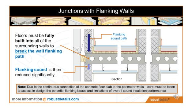
Sound energy can get into the structure, and flank around the edge of the floor.
