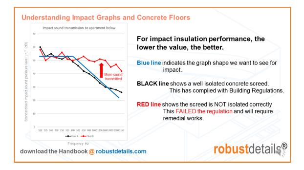
As mentioned in previous modules - for impact sound insulation – we measure the amount of impact noise transmitted from a standard tapping machine (Y-axis) for a range of frequencies 100Hz to 3150Hz (X-axis). The lower the value the better the impact insulation performance. The Blue line gives an indication of the type of shape we want to see for an impact graph.
