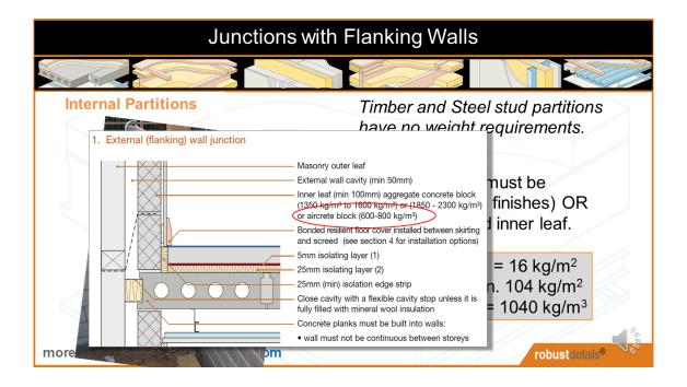
Lightweight structures don't have any minimum mass requirements, but when we start combining masonry partitions with concrete floors – or indeed masonry separating walls, the partitions can start transmitting noise into the structures. So Appendix A1 says the partition has to be a min.120 kg/m<sup>2</sup> (incl. finishes) OR that of the approved inner leaf.
