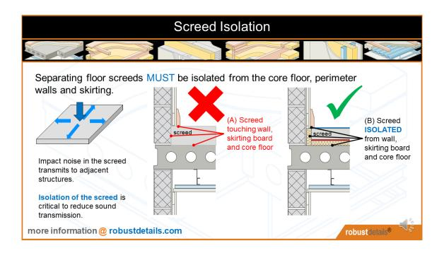
Separating floor screeds MUST be isolated from core floor and perimeter walls and skirting
