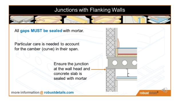
Where concrete floor slabs are built and rest on the wall head no gaps should remain and the joint MUST be sealed with mortar.
