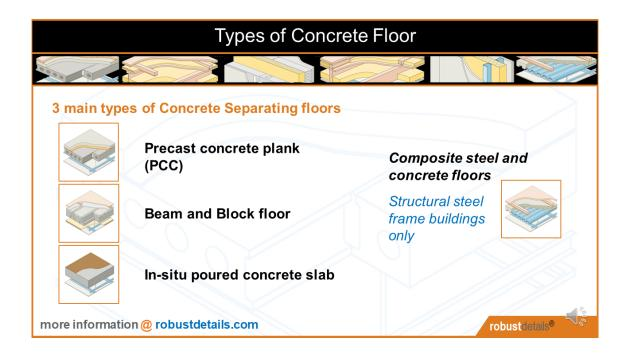
There are 3 types of concrete floor that are in general use in Robust Details. These are: <as slide>
