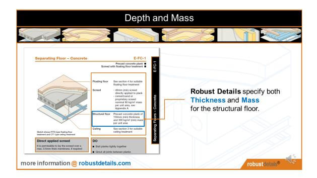
Robust Details specify both Depth & Mass in order to give the required sound insulation performance.
