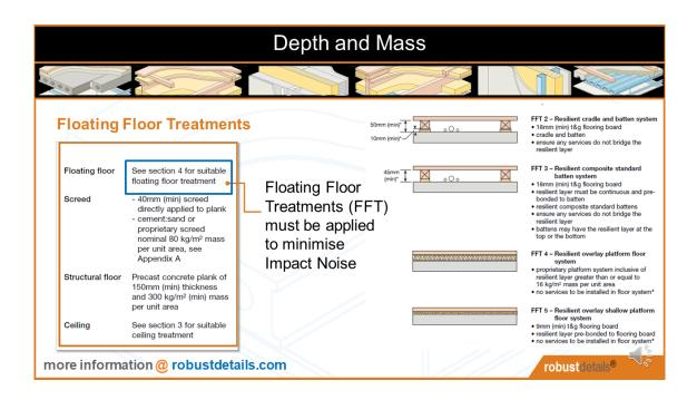
Impact noise, from people walking in the apartment or flat above, needs to be addressed by using a floating floor treatment, or FFT.
