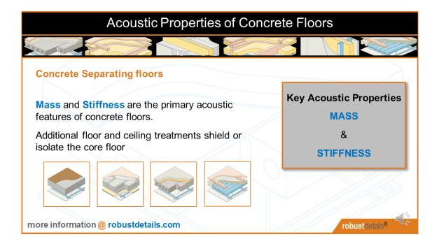
MASS and STIFFNESS are the primary acoustic features of concrete floors.
