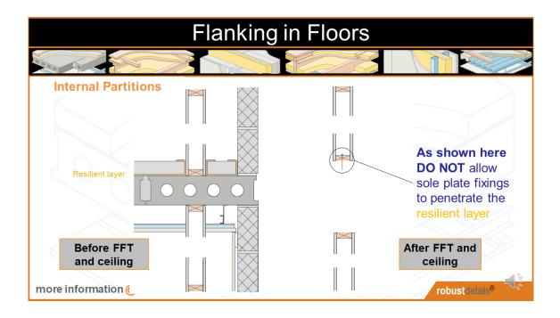
Partitions can be fitted direct to the structural floor, so no resilient strips necessary – and then the FFT and ceiling can be installed. So that impact noise doesn't flank through, ensure the screed is fully isolated from the partition, the same as it would be from any other wall. Same for the ceiling – ensure there are no air-paths up into the ceiling void.
