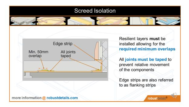
It is critical that the resilient system, comprising the resilient layer and flanking edge strips, are properly installed with the required overlaps – and tape is securely applied.
