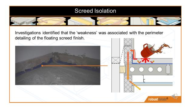
During the Robust Details monitoring, an impact fail was recorded – and the weakness was narrowed down to the perimeter.
