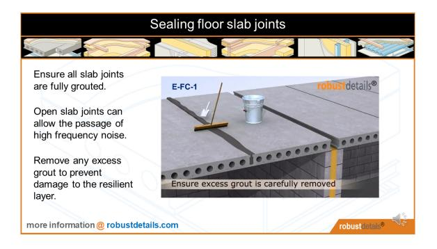
Ensure all joints and gaps in the planks are fully grouted. This enhances the floor stiffness, and stops the passage of high-frequency noise.
