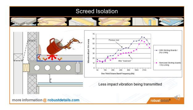
After the remedial works and with the skirting still off, another measurement was taken, which showed a 7dB improvement - so if the job was done right to start with, this would have been a good 57 dB pass, well below the 62dB maximum requirement for Part E and max 60dB for RD impact performance.
