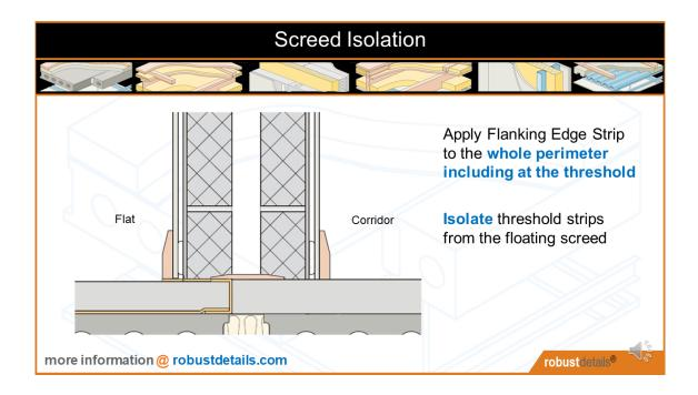
The Robust Detail specifies that the flanking edge strip must be applied to the whole perimeter of the floating screed – so this includes at the threshold of the entrance door.
