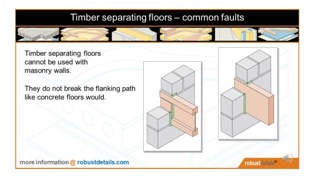
As stated at the top of page 1 of each of the timber separating floors, they are for "Use with timber frame walls only".
