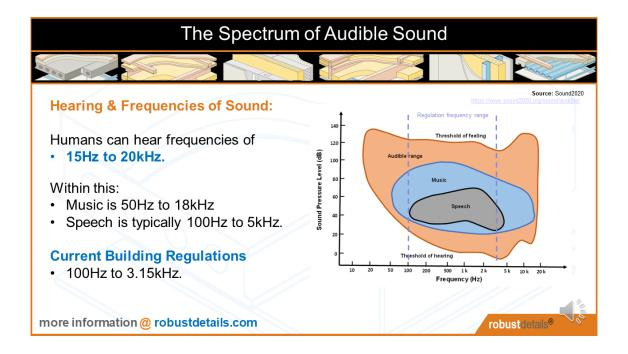
The audible frequency range of humans typically ranges from 15Hz to 20kHz. With aging process as early as 30 years our frequency range can decrease.
