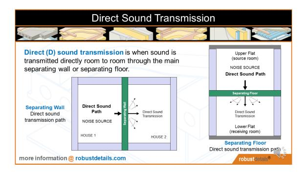
Direct (D) sound transmission is when sound is transmitted directly room to room through the main separating floor.
