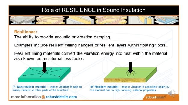
Resilience: Is the ability for materials or products to provide an effective acoustic or vibration damping. Often involving a combination of acoustic factors such as absorption and the ability to retain their shape and form, but also to dynamically absorb displacement forces. Examples include resilient ceiling hangers or resilient layers within floating floors, under-screed layers and bonded soft floor coverings, which absorb impact vibration from footfall.
