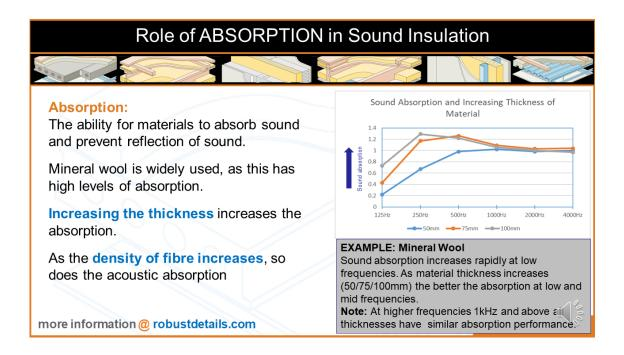
Absorption: Is the ability for materials to absorb sound and prevent reflection of sound. This is commonly used to improve airborne sound insulation. Materials such as mineral wool have high acoustic absorption.
