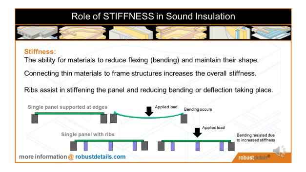
Stiffness: Is the ability for materials to reduce flexing (bending) and maintain their shape. If a construction material is too thin or the structure of the materials allows bending to occur, then this leads to flexural movement. Thin panels such as gypsum board or plywood will more easily flex. Connecting such materials to frame structures such as timber studs or joists reduces the flexibility and increases the overall stiffness. Double linings (e.g. gypsum) increase wall panel stiffness.
