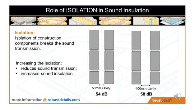
Isolation: The isolation of construction components can break the transmission of sound.
