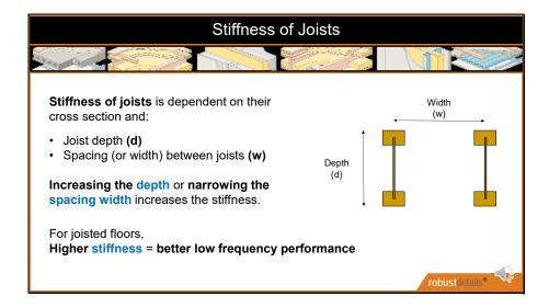
Stiffness of joists is affected by the material cross section and two key factors:
