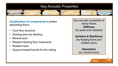
Timber separating floors involve a combination of components to deliver the required sound insulation.
