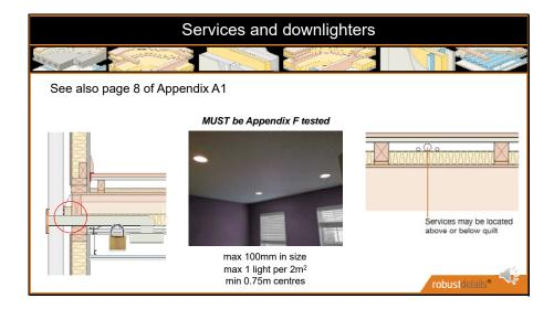
As we can see here, we need to have blocking between the joists to prevent flanking noise transferring between the external cavity and joist zone
