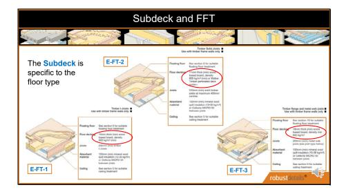
Each of the Robust Details timber separating floors will include a subdeck specification and they will vary from floor to floor.
