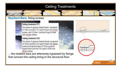
The ceiling lining on timber separating floors always comprises 2 layers of gypsum board, and these could be the same, or different thicknesses
