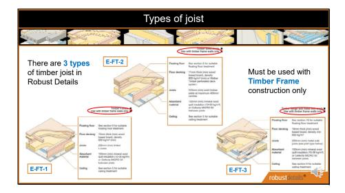
The Robust Details timber separating floors use three different types of joist, as we can see in these generic floors.
