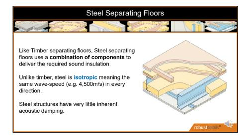
Steel separating floors are very similar to timber separating floors involving a **combination of components** to deliver the required sound insulation.
