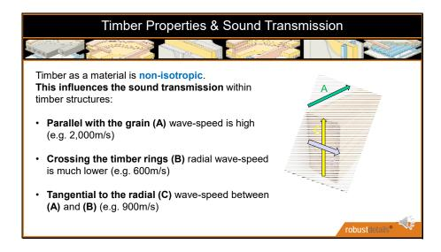
Timber as a material is non-isotropic. This means that the material properties vary depending on the direction of the grain. This in turn influences the sound transmission within timber component structures.
