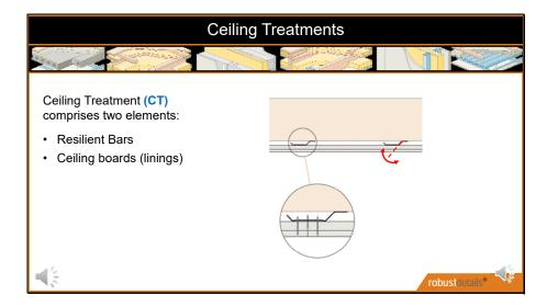
Ceiling treatments are made up of 2 parts: Resilient bars; and the ceiling lining itself
