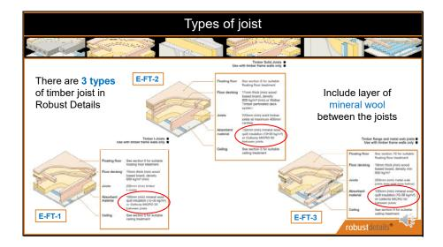
We also need to ensure that the specified mineral wool is fitted in the joist zone
