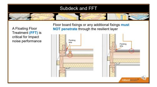
The floating floor treatment is an essential part of the floor build-up. As well as adding to the airborne performance, its primary function is to contain impact noise, and reduce it from transmitting into the structure, and into the flat below.
