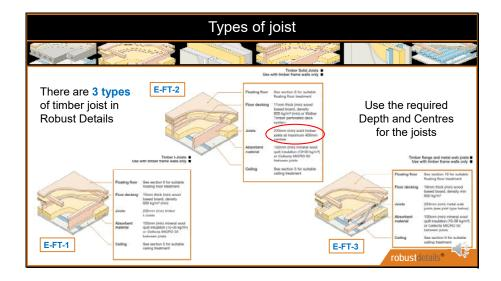
With no inherent mass to address the mid to low-frequencies, these floors have to rely on their acoustic stiffness.
