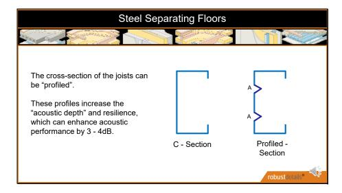
To increase the effective "depth" of a steel floor beam and improve sound insulation performance, the cross section can be profiled as shown here.
