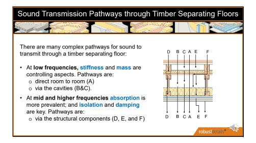
There are many complex pathways for sound to transmit through a timber separating floor:
