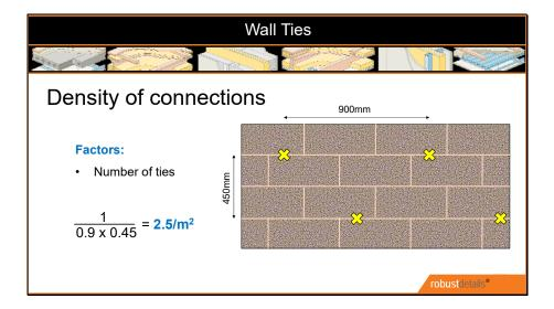
The third part of the equation is the number of connections – or number of ties. As we all know, the standard spacing for the ties is 900mm horizontally, and 450 vertically
