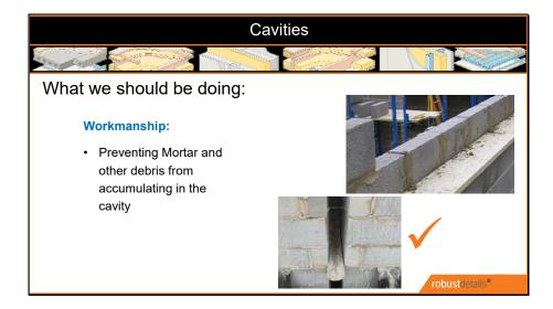
We could look to clean the mortar off the ties; and clear the base of the cavity every couple of hours,
