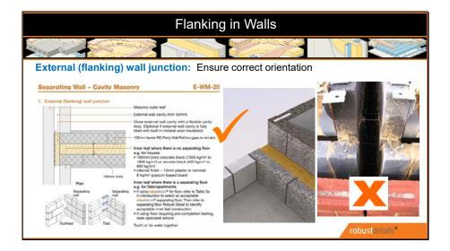
Here we see the end of an aggregate separating wall as it meets an aircrete inner leaf.
