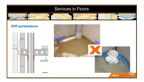
Where SVPs or other services pass through the separating floor, part of the floor structure has to be removed, which introduces a weakness. So we need to shield, or protect the hole in the floor
